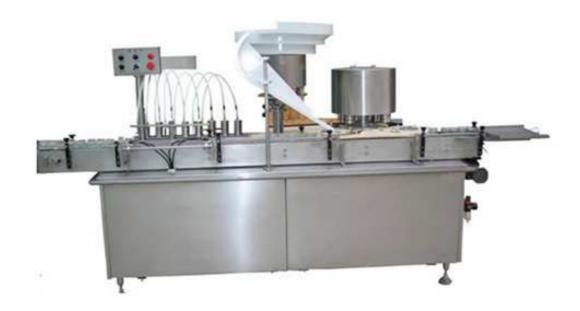
This machine is the main filling equipment of the liquid filling production line, which is mainly applied in the filling and sealing of 30 – 500 ml glass bottle or plastic bottle.
