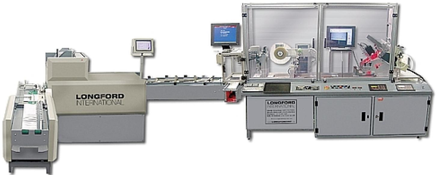
Design/build a Custom Cheque Return System. Provide a custom turnkey line that feeds and image captures each cheque and matches it with the client control sheet. Band each package using a shrink band and transfer it into a third party envelope system.
