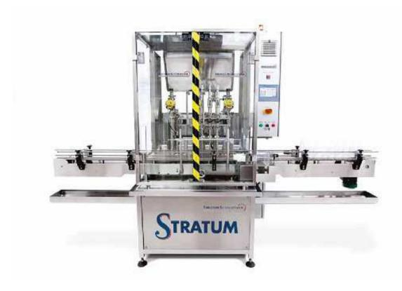
Applicable to containers of most common shapes and sizes in the food & beverage, chemicals and cosmetics industries, STRATUM has servo driven piston technology at each filling station, which significantly lowers utilities consumption and reducing costs while boosting portioning accuracy levels.
