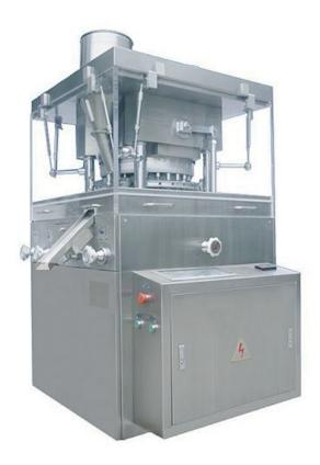
That machine is a double press automatic rotation for shape-pressing equipment, which have the function of press the grains material to be round or irregular shape tablets, such as candy, calcium tablets double-sides with letter printing and etc. which widely suitable for the Industries of pharmaceutical, Chemical, Foodstuff, Plastic Electronic, Powder Metallurgy and so on.
