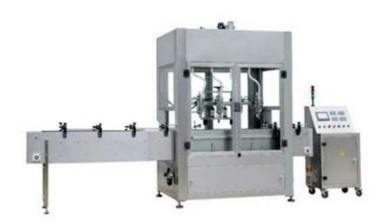
The machine adopts PLC programmable control system and weighing feedback system to realize quantitative filling. Applicable to pesticide, chemical, chemical industries and no bubble water fluid filling.
