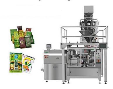
Full Auto Vacuum Rotary Packing Machine is a new product which self-developed by our company. This machine can use manipulator to automatically get vacuum bags, open bags, print date or batch number, feed products, vacuum packing, etc. so that can be with no-man operation and can do fully automatic package. Bag length can be 100-240 mm, width can be 70-140mm.
