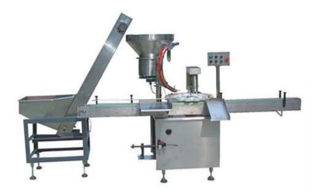
This wide-mouth bottle screw capper is specially designed for capping wide-mouth glass and plastic bottles, and the elevator is used for feeding caps. And its main components are elevator, capping system, and control system.
