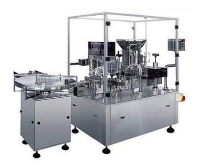
FG-KFS2-B type powder filling machine is a kind of screw type sterile powder filling machine our company has newly developed. It adopts two track, cylinder positioning, 2 head screw filling and 2 roller stoppering. The servo motor controls the filing auger precisely.
