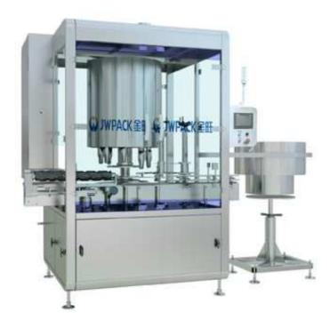
This machine is suitable for automatic compression of glass or plastic bottles. The whole machine is a rotary structure, with the vacuum suction nozzle absorbing various inner plugs transported by the scraping cover plate, and closing the inner cover during the bottle rotation process. The whole machine adopts PLC control, touch-type human-machine interface, convenient and intuitive operation.
