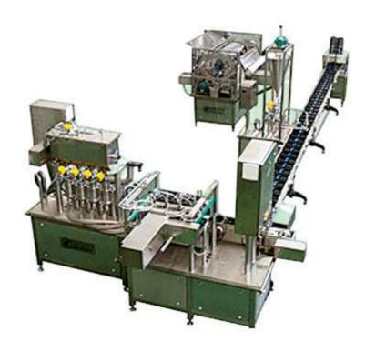
**Performance:** Automatic PAO-SQ Line of machines performs membrane cutting and sealing from the roll.
