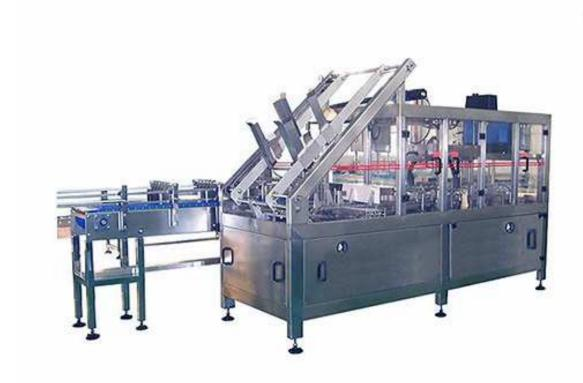
GF1509 Wrap Around Carton Packing System can finish the process of the cardboard sucking, product Packing and carton forming.
