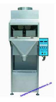
It is used in powder, aginomoto chicken powder, salt, rice etc grain product ration packing machine.
