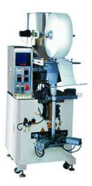
Able to automatically complete discontinuous running of measure, filling, counting, printing (it is necessary to separately configure coder), merging functions of photoelectric trace and step-less speed regulation into a single whole with finished products as triangle, which is very novel and unique.
