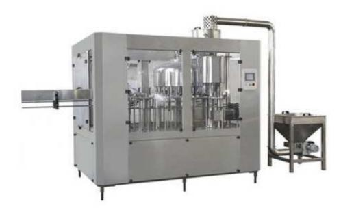
The machine is a full-automatic multiple-function washing, filling and capping unit. It is used in washing. filling and sealing all kinds of non-air drinks such as fruit juice, oil & vinegar, wine, fruit wine, mineral water and pure water. The line has features of unique design, new style, complete functions, multi-purpose, convenient in operation, beautiful construction, high automatization. It is the best filling equipment in China.
