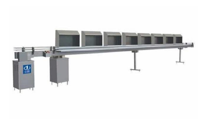
SDPJ500 equipment is used for visual inspection using a light shade of glass bottles for infusion solution after the sterilization process. The number of light stations is a dependence on the performance of the processing line. This equipment is suitable for bottles and vials of 50 ml, 100 ml, 250 ml and 500 ml. Due to the wide range of performance from 30 to 600 bottles per minute, this machine meets a variety of production requirements. Electrical power is 3.3 kW.
