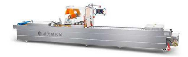
Thermoforming (from wikipedia.org) is a manufacturing process where a plastic sheet is heated to a pliable forming temperature, formed to a specific shape in a mold, and trimmed to create a usable product. The sheet, or "film" when referring to thinner gauges and certain material types, is heated in an oven to a high-enough temperature that permits it to be stretched into or onto a mold and cooled to a finished shape. Its simplified version is vacuum forming.
