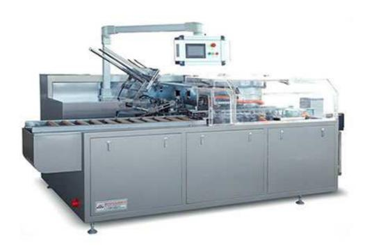
The KXZ-450C cartoning machine is an intelligent packing machine with a packaging speed of 80 cartons per minute. The machine can be applied to package preservative film, aluminum foil rolls, napkins, and other consumer goods. It is suitable for packages of 100-450mm in length, 20-80mm in width and 20-90mm in height while special sizes can be customized.
