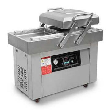
DZ-400/2SB vacuum packaging machine can finish the whole programs of vacuum extraction, inflatable device (optional), sealing, cooling and exhaust automatically. The products after packing can be prevented from oxidation, going mould, insects or getting damp, thus can be kept fresh for longer time. This is an efficient, sustainable double chambers model for outstanding vacuum packaging results.
