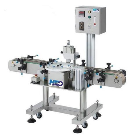
Automatic Vial Crimper NCP-300 is designed for capping aluminum caps. Its inline structure with star wheel bottle spacing system makes the crimping process more efficiently. To promote productivity, an automatic cap feeding system is also available as an optional accessory.
