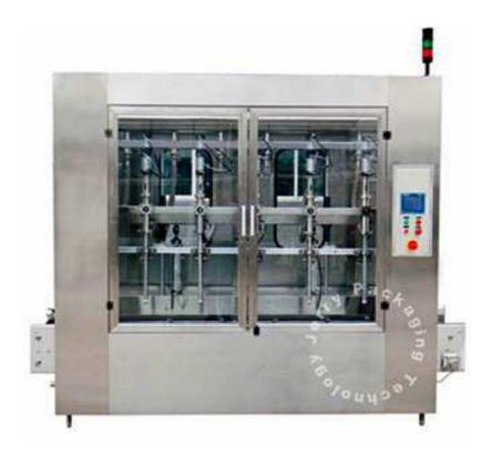
JWF Series Scale Fixed-quantity Filling Machine is making up of the scale (with roller), chaindriven drum in and out structure, fast and slow filling (with dive function), material tank, weight control meter and PLC control unit.
