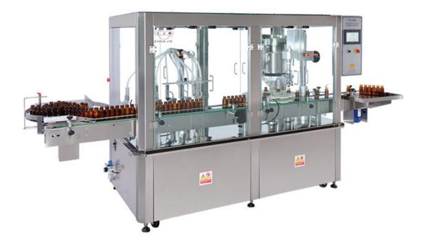
The liquid packaging equipment compliances with cGMP liquid production guidelines and the common application is for above 60mL low viscosity products.
