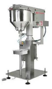
Independent drive through motor controlled by electronical speed inverter, Independent stirring rods, Auger dosing implements provided with "clapet" closure to avoid leakages, Supply funnel level, in order to control the devices of the product supply to the dosing unit, Weighing platform equipped with weight cell, Control box equipped with CPU microprocessor provided with the following applications:
