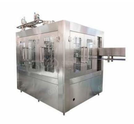
This machine works harmoniously with air-conveyor belt, It holds the bottles by the neck, thus, reducing the possibility of bottles falling over during conveying process. This machine is used to fill still water into pet bottle and with screw caps capping function.
