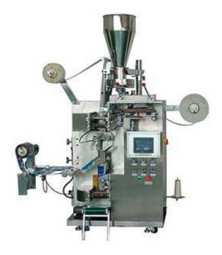
This tea bag packing machine has an automatic device instead of an envelope packing system. It is an automatic precision machine use for packing broken tea and similar herbs into small bags and realize fully automatic procedure including ration filling, heat sealing of tea bag, pasting thread, linking tag, dividing groups and counting tea bags.
