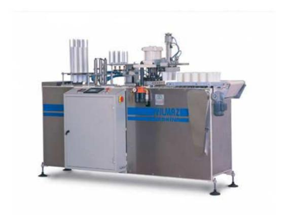
IA full automatic glass filling machine. It is a practical, fast packing machine produced with the latest technology.
