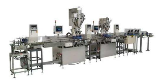
PF3 is the linear transport type Auger Filling System. It is also possible to build up a high accuracy filling system by adding a correction filling station after the initial filling. There are variety of optional devices to make your complete production line, such as container feeding, capping machine, labeling machine etc.
