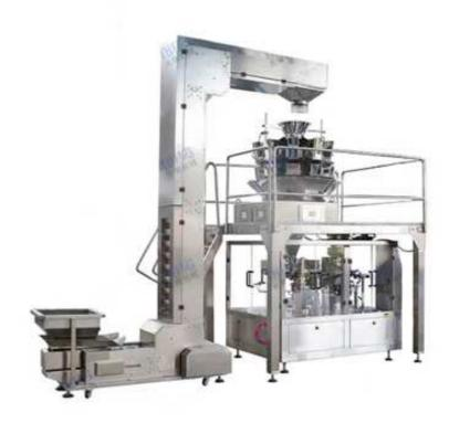
This premade pouch packing machine is widely used in solid particles of various shapes with good fluidity. Such as nuts, seeds, popcorn, potato chips, snacks, mini-cookies, biscuits, red date, peanuts, candy, pet food, and many kinds of hardware's.
