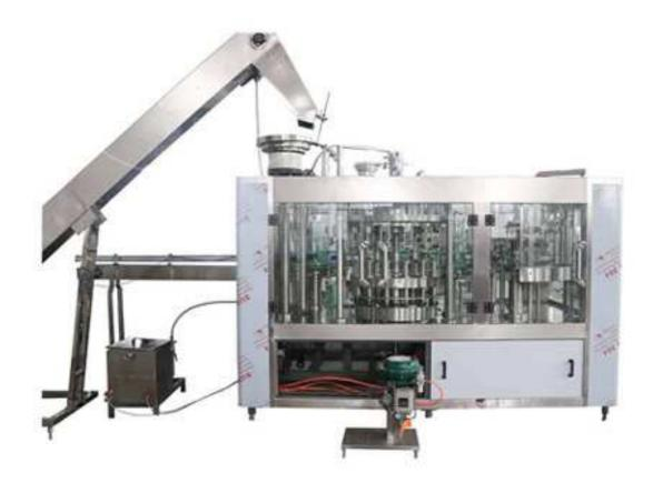
Our newly designed BCGF serious monoblack beer filling machine is designed for bottle filling, it can suit for PET bottle and glass bottle and aluminum bottle, size between 150ml to 2000ml, can customized to maximum of 3000ml. Genus design of capping design makes different screw cap change into one simple easy torch. On machine surface is only leaving 3 points of bearing support point which makes drainage so easy and without any dirt stain.
