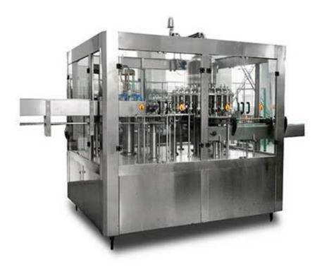
The series Drink filling machine is used for bottle rinsing and hot filling and sealing 3-in-1 unit machine for green tea, black tea, wulong tea and fruit juice. And with only a few parts changed, the machine can also be used for mineral water or pure water drink filling.
