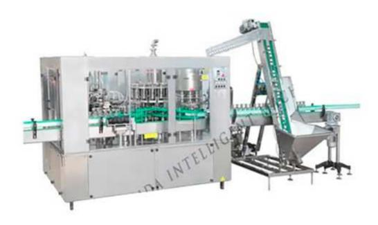
PET Bottle Juice Filling Machine can be used for making orange juice, apple juice, peach juice, cherry juice and most common commercial juice. The raw material could be fresh fruit or concentrated juice. We also can design custom production lines accordance to customers' requirements.
