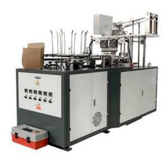
PT-480 automatic take-out box food tray forming machine is designed to erect and form paper box like take-out box, food tray, lunch box, fruit tray, etc.
