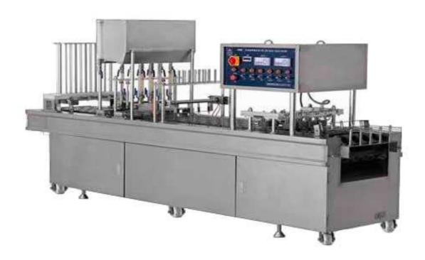
BG series automatic plastic cup filling and sealing machine with code printing, plastic box automatic capping machine, plastic cup filling, sealing, and printing machine
