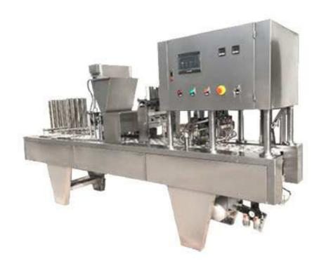
Linear Coffee Capsule Filling & Sealing Machine is automatic high-speed sealing machine. From drop cups, filling, put the film, print dates, twice sealing to out are all automatic operation. The electrical and pneumatic components are all using famous brands (can be also customized by customers' requirements), with stable quality, long life. It is mainly used in the products packing like: coffee powder, milk powder, rice, wheat powder and so on.
