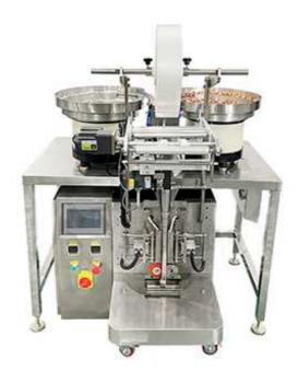
This machine is designed for quantitative packaging of small items such as screws, hardware accessories, plastic accessories, etc. It is widely used in hardware lighting, furniture, screws and other industries. The overall structure of the equipment should be reasonable, firm, beautiful, reliable and durable.
