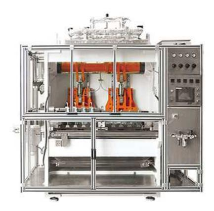
XLD Series Vertical stamper is equipped with servo control and cam system, reliable and accurate. Control system adopts world famous brand PLC and servo, touch screen and electrical hand wheel, which makes it for operation and adjustment. This machine uses Germany FESTO and Japanese SMC pneumatic elements. It has complete covers with safety door switches to ensure operators' safety.
