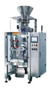
DXDL42 Vertical Packaging machine is to pack bulk granular or powdery material into small bag.It can realize full-automatic packaging through metering, bag forming, coding, filling, sealing and other functions. This model is suitable for pillow bag and has a special design for powerful corrosion working circumstances.
