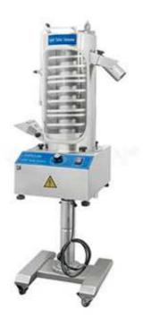
Uphill Tablet Sieving Machine SZS230 is developed by absorbing advanced technology at home and abroad. It has the dual functions of tablet improvement and dust removal so that it can work in conjunction with various tablet pressing machines and metal detection machines. This machine can be applicable in the field of pharmaceutical industry, food industry, chemical engineering, electronics, and so on.
