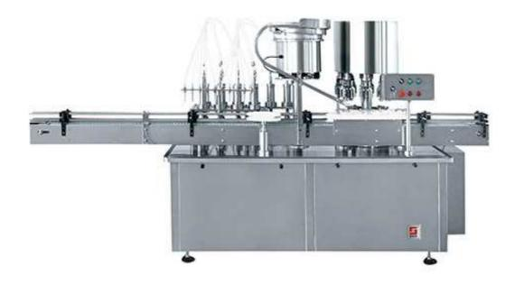
Suitable for filling and cap screwing (capping) for glasses and plastic bottles from 30ml to 500ml.
