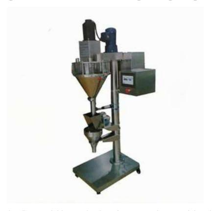
It can be adapted to the direct weighing packaging of most powder materials, which can effectively solve the problem of material packing of cotton, sugar tea and other relatively large humidity.
