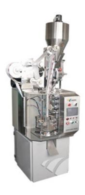
Model DXDC50 Pyramid / Triangle tea bag packing machine is our new pyramid tea bag packing machine, and it could use the non-woven fabrics and nylon filter fabric to produce pyramid bags which have good perviousness and perspectivity. It is used for the packing of tea leaves, such as green tea, black tea, etc. And it is also used for the pyramid bag or flat bag packing of food spice whose taste exudes through bags.
