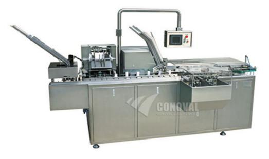
DC100H Automatic Cartoning machine applies to the encase packing of blisters, vials, cosmetics, poker and similar stuff. This machine can fold leaflet, open carton and insert stuff with leaflet into cartons, printing batch number and close carton automatically.
