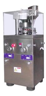
The machine is a single-press type, continuous automatic tablet press for pressing granular raw materials into tablets. It is used for small-scale production.
