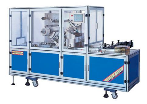
This machine is designed and developed on base of absorbing the advantages from the same product abroad, it is a product integrating mechanical, electrical, and pneumatic, to be stable running, smooth and tight sealing and convenient, advanced, beautiful technical and operate easily. It is composed of aluminum alloy rack and organic glass safety guard, which is used for packing middle single box.
