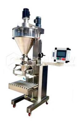
This Semi-automatic pouch filling machine is OEM designed for our Europe Agent. It can be applied to the quantitative measurement of a variety of powders or fine particles with big dosing 10-25kg such as flour, coffee powder, milk powder, tapioca flour, seasoning powder, chemical powder and other materials. By linking screw conveyor, Sewing machine or Heat sealer, it could set up a semi-auto powder packing line for the open-mouth bags.
