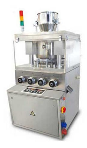
ZP45 rotary tablet press machine is a new generation product. It is a double-press type, continuously automatic rotary tablet press for pressing tablets. It is widely applicable to industries such as pharmaceutical, chemical, foodstuff, electronic and etc. for pressing the granular material into all kind of round tablets, irregular tablets, two colors tablets and ring shaped tablets.
