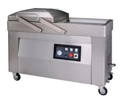
Double chambers vacuum packaging machine can complete the set programs of vacuum extraction, gas flushing (optional), sealing, printing, cooling and exhaust automatically. The products after packing can be prevented from oxidation, going mould, insects or getting damp, thus can be kept fresh for a longer time.
