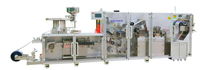
According to different packaging materials and principles of forming, Blister packs may be divided into mainly two types: aluminum/plastic (thermoforming) blister pack and aluminum/aluminum (cold forming) blister pack.
