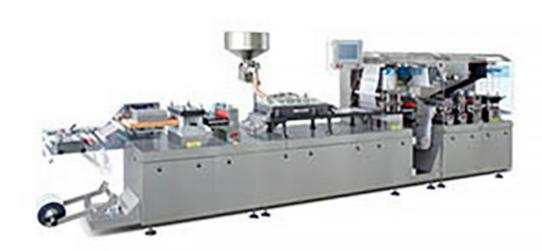
DPP-300KII Aluminum Plastic/duralumin Packing Machine with advanced performance, simple operation, high output is the latest improved equipment in our company. It is the best ideal packing equipment for large and medium-sized pharmaceutical plant, health care factory and food industry.
