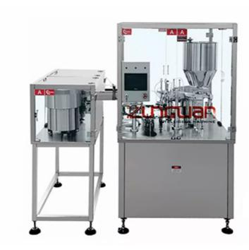
ZHGX-60EM Type machine is designed for suppository tube filing and capping. The machine can finish the whole packaging progress of automatically unscrambling, filling, cap sorting, cap feeding, capping and finishing product outlet.
