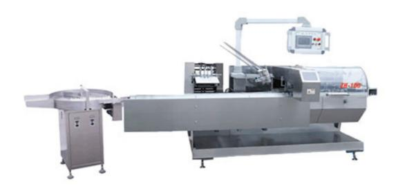
ZH-100P Automatic Horizontal Cartoning Machine for bottle used for packing all shape of bottles and similar good into cartons including automatic leaflet folded, cartons open, feeding, embossing and sealing. etc. Also can adding hot-glue device extra. Adopt PLC control and photoelectron to easy to solve troubles.
